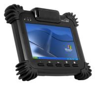
With IP54 and MIL-STD 810G ratings, the WebDT 372 provides protection from water, dust, and shock vibration. An option for outdoor viewable screen and Bluetooth and Wi-Fi connection contributes to truly anywhere operations. The Intel® Atom™ processor gives high performance with low power consumption, and support for Microsoft® Windows® or Linux operating systems add to the flexibility of integrating with other applications and systems.
